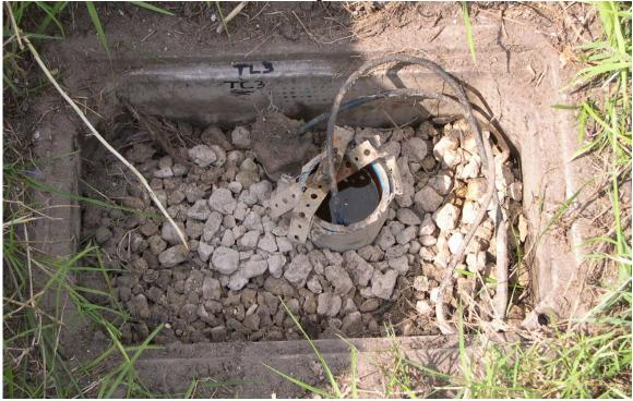
Soil Tiltmeter 3 removed from its slotted inclinometer casing
